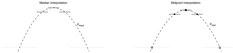
Fig. 2 The rules for the nonlinear median-interpolating subdivision scheme (left), and the linear midpoint-interpolating scheme (right) are close but not identical.
